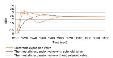
Note: Values measured during testing with the EEV are always higher than the EER values measured using the TXV, with or without a solenoid valve. This higher energy efficiency is ensured by the EEV's capability to optimize the control of refrigerant flow in the evaporator, thus limiting the delivery of liquid into the compressor.
