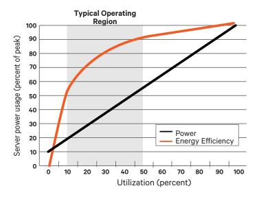
Source: Hölzle, 2017. Note: In a more energy-proportional server (red line) the power efficiency is more than 80% of peak value for utilizations levels of 30% or more with efficiency remaining above 50% for utilization levels as low as 10%.
