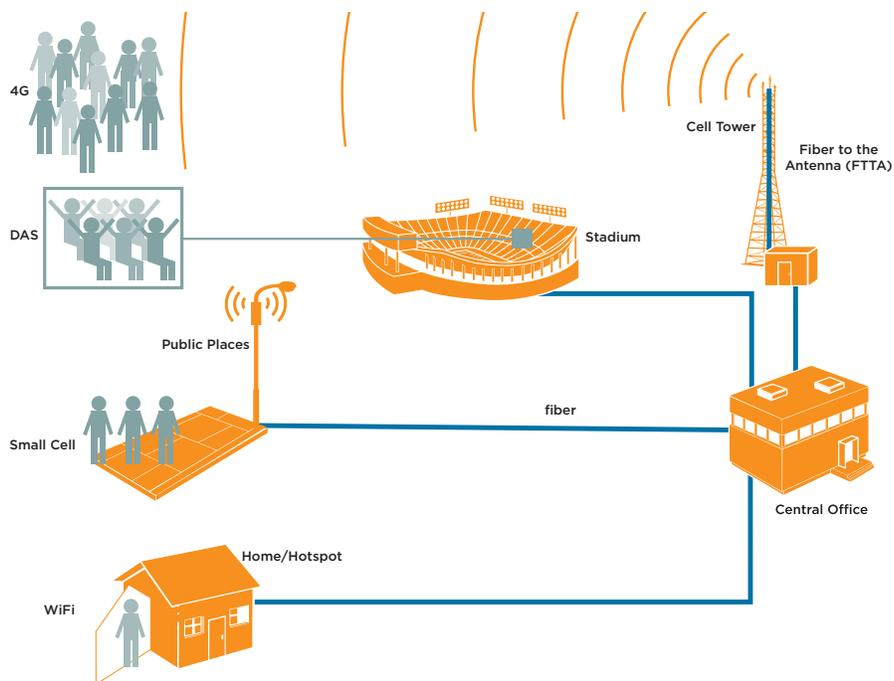
Figure 3: Wireless is a heterogeneous network comprised of 4G macrocells, DAS (Distributed Antenna System), small cells, and WiFi hotspots for maximum coverage and capacity.
